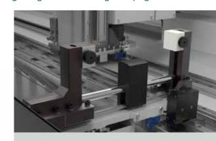
To extend the clamping capacity and the working areas, cast iron EXTRA CLAM-**PING VICES** are available, in which closing of the jaw is carried out using straight guides.
