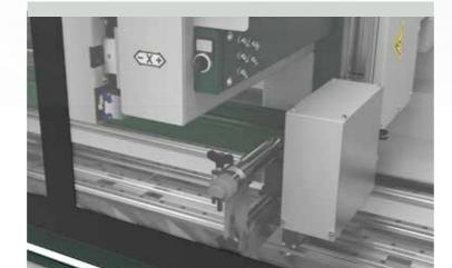
MACHINING HEAD allows machining operations to be carried out on 3 sides of the profile at any angle between 0° and 180° and on the 2 ends. The brushless motor allows exceptional performance in terms of acceleration and speed, placing the FMC 230 at the top of its category.
