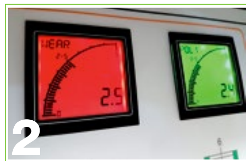
Digital ammeters and polishing wheels automatic wear detection system
