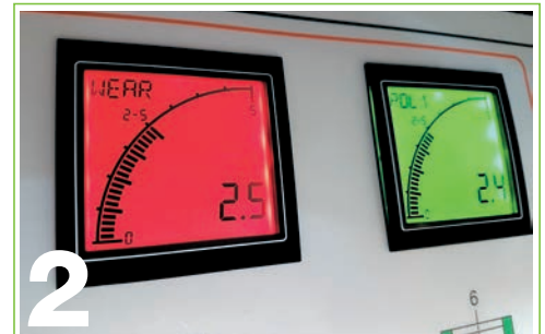
Digital ammeters and polishing wheels automatic wear detection system
